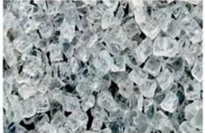
tempered glass broken with very strong external force cubical debris will fall down
