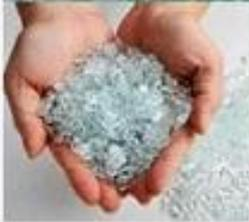
**Toughened (tempered) glass breaks into many small pieces with less sharp edges.**
