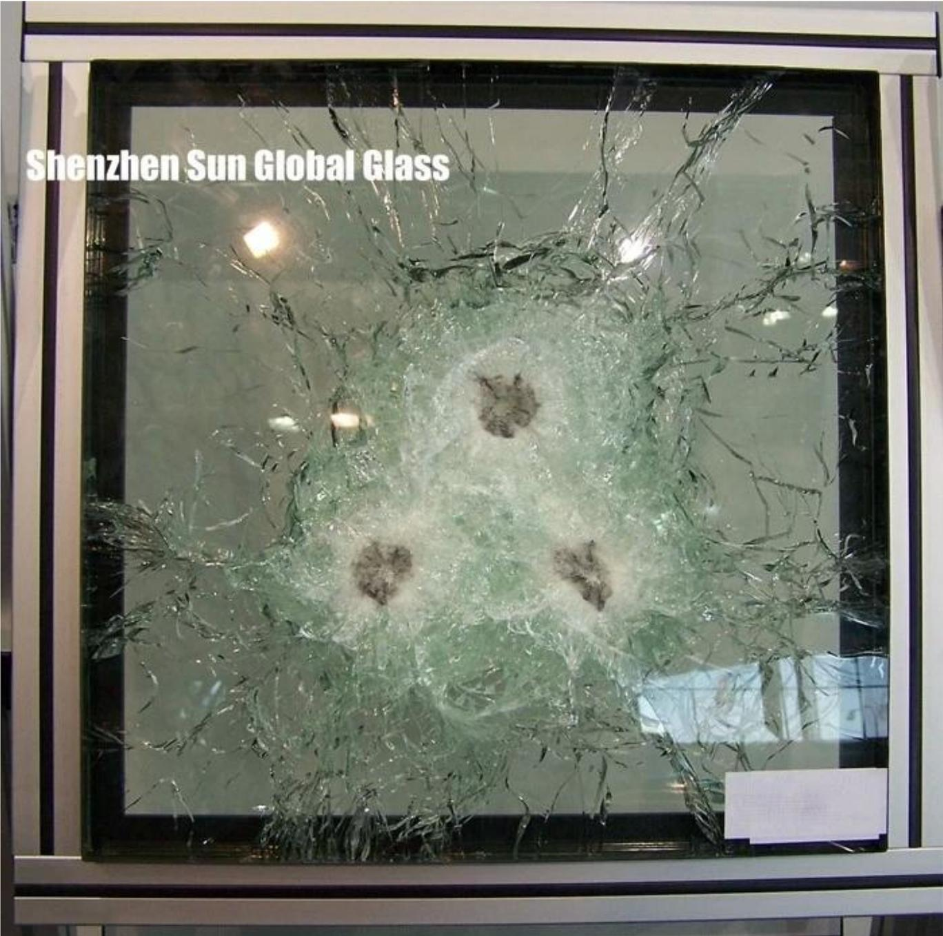
A photograph of a rectangular piece of laminated glass that has been shattered. The glass is held together by a dark frame. The shattering is extensive, with many sharp, jagged fragments of glass still attached to the central pane. Three distinct, circular impact points are visible, each with a dark, irregular hole in the center. The background behind the glass is a light-colored wall with some reflections. The text "Shenzhen Sun Global Glass" is overlaid in the top left corner.
