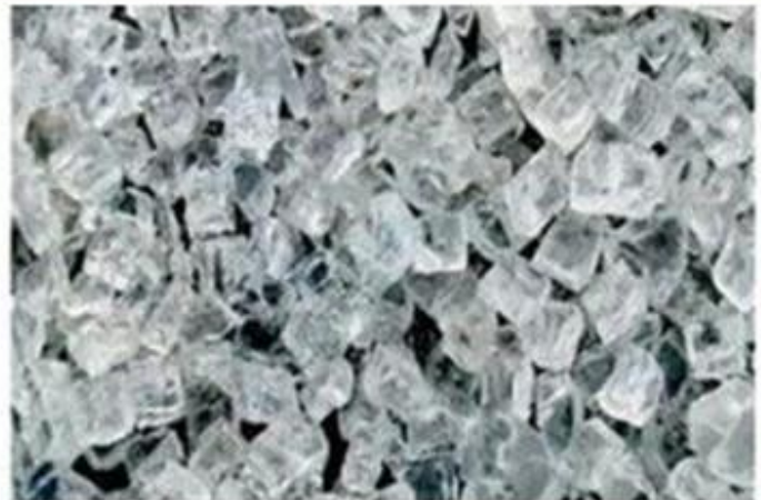
tempered glass broken with very strong external force cubical debris will fall down
