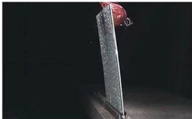
SGP laminated glass impact test
