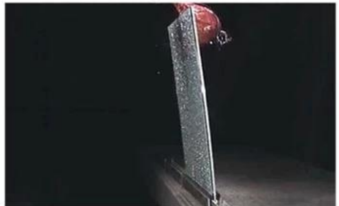
SGP laminated glass impact test
