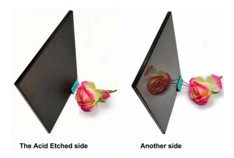
Sun Global Glass produce 10mm bronze acid etched tempered glass by using the best quality bronze tinte d glass to hydrofluoric acid process that make the surface of glass has a a frosted look. After acid process, the glass will put into tempering furnace to process the glass into <u>tempered glass</u>.
