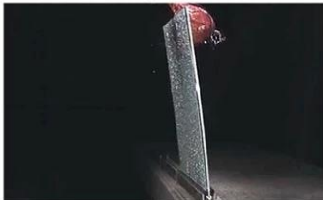
SGP laminated glass impact test
