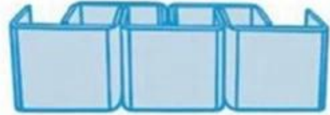
双排 翼错开排列 Double glazing Stagger arrangement
