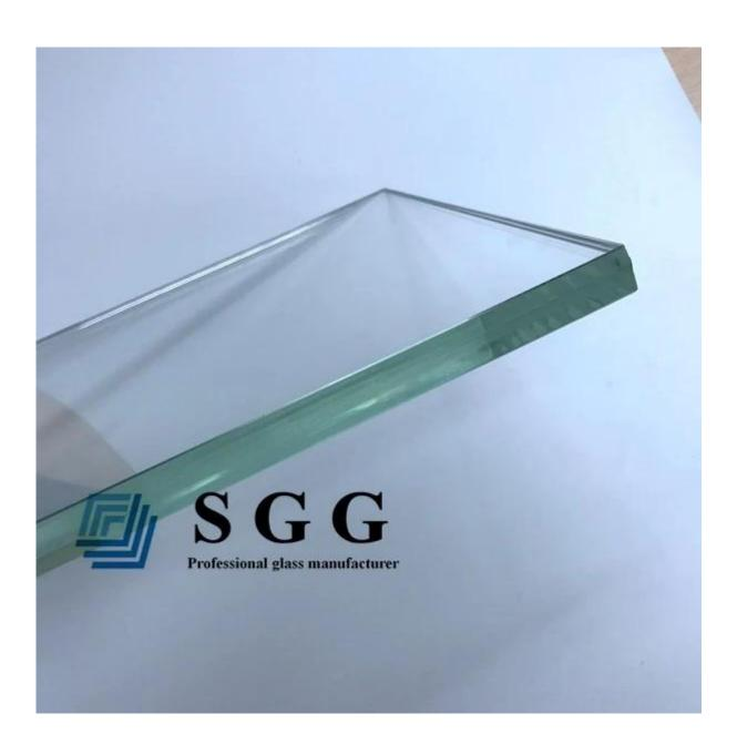
In this section, 8.89mm SGP tempered laminated glass are applied for shower glass doors, shower enclosures, etc., they are produced by <u>4mm clear tempered glass</u>+0.89mm SGP film+4mm clear toughened glass.
