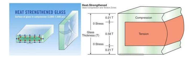
Heat-strengthened glass is annealed glass that has been heat treated to have a surface compression between 3,500 and 7,500 psi (24 to 52 MPa) which is twice the surface compression of annealed glass and meets the requirements of ASTM C 1048.
