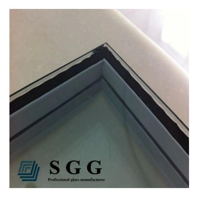
From here you can have very flexible combinations of warm edge spacer IGU, such as: 6MM THK. HS CLEAR TEMPERED GLASS + 15MM A. + 6MM CLEAR GLASS WITH LOW-E COATING #3 + 1.52 PVB FILM+ 5MM H.S. LAMINATED GLASS, 6mm LOW-E TOUGHENED GLASS/16a/TEMPERED GLASS 4mm/16a/LOW-e 4mm TEMPERED GLASS, 5MM TEMPERED GLASS+6A+5MM CLEAR TEMPERED GLASS, etc.
