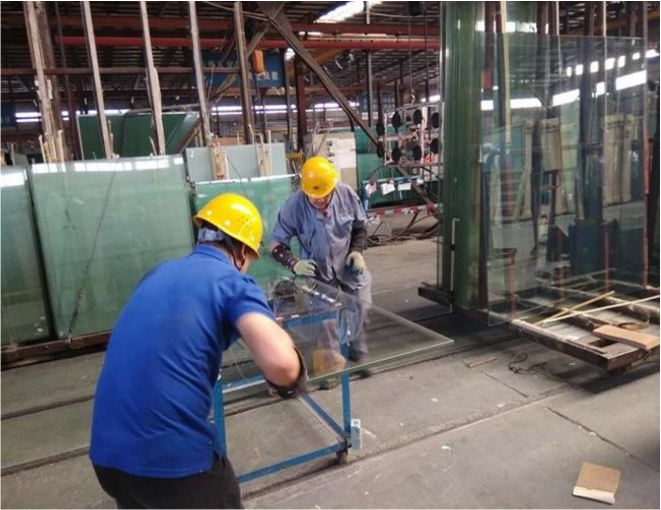
The processing of tempered laminated glass
