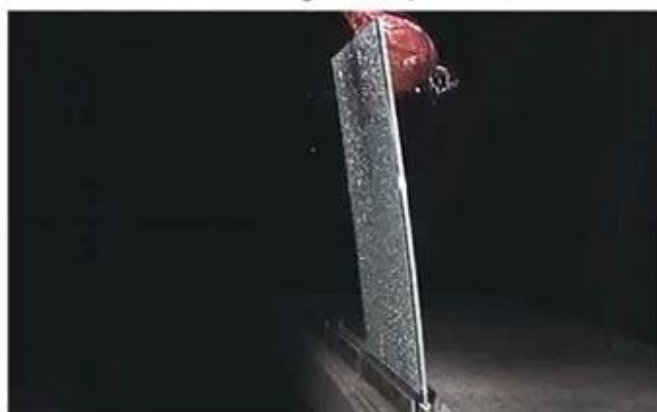
SGP laminated glass impact test
