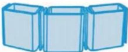
Double glazing Arranged in zig-zag formation in pairs
