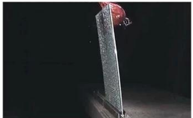
SGP laminated glass impact test
